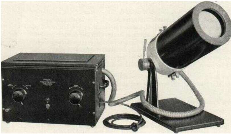
The General Radio Cathode-Ray Oscillograph for table mounting. At the left is the TYPE 496-AM Power-Supply Unit; at the right, the TYPE 497-A Tube Mounting containing the tube
